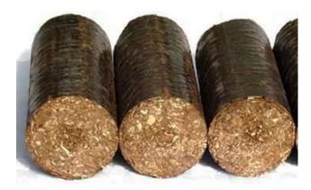
Biomass Briquettes in Kenya are made from bio-degradable waste materials such as saw dust, coffee husks, rice husks, bagassee, tobacco dust and hay.
